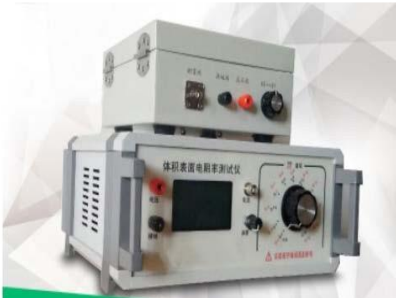
Insulation resistance test 1台
